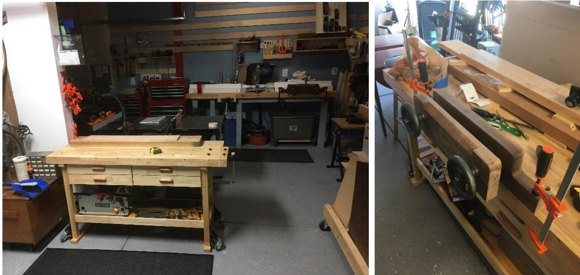
I made the Moxon-style vice (above right) with purchased hardware and hand-shaped the jaws out of walnut. It offers the advantage of being a very flexible and strong holding device that I can clamp to any of my benches or tables to get the working height needed for planing and for cutting joinery such as dovetails (below left) without wrenching my back.
